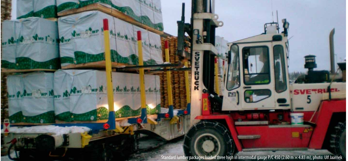
Standard lumber packages loaded three high in intermodal gauge P/C 450 (2.60 m x 4.83 m), photo: Ulf Jaarnek
